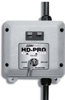
TRC engineers designed the HD-PRO models specifically for high current, rugged environments and these models are field-proven in all kinds of tough applications. The entire HD-PRO family (120V/30A to 600V/80A) is designed to trip within 25 milliseconds after ground fault detection at an adjustable selected trip level of 6, 10 or 30 mA.
