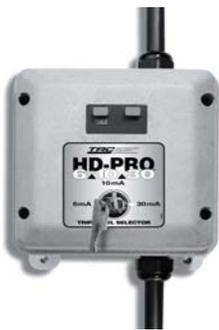
TRC engineers designed the HD-PRO models specifically for high current, rugged environments and these models are field-proven in all kinds of tough applications. The entire HD-PRO family (120V/30A to 600V/80A) is designed to trip within 25 milliseconds after ground fault detection at an adjustable selected trip level of 6, 10 or 30 mA.
