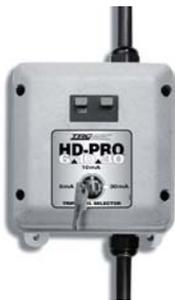
TRC engineers designed the HD-PRO models specifically for high current, rugged environments and these models are field-proven in all kinds of tough applications. The entire HD-PRO family (120V/30A to 600V/80A) is designed to trip within 25 milliseconds after ground fault detection at an adjustable selected trip level of 6, 10 or 30 mA.
